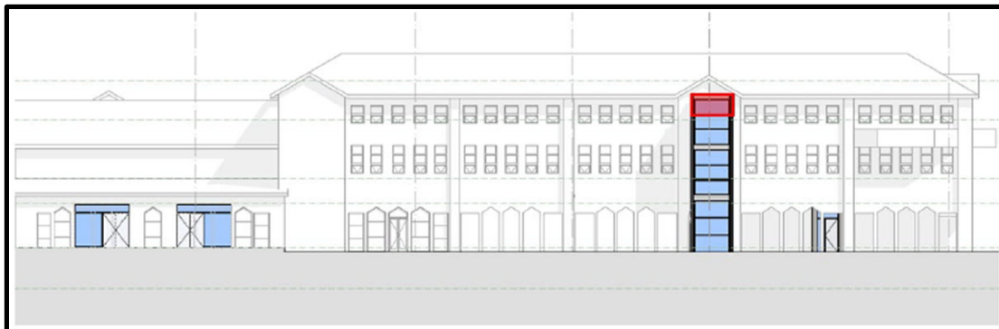
Figure 9 Proposed Rear Elevation of Block F (Non-Conforming Lift Shaded Red) (source: DFP Planning Pty Ltd)
