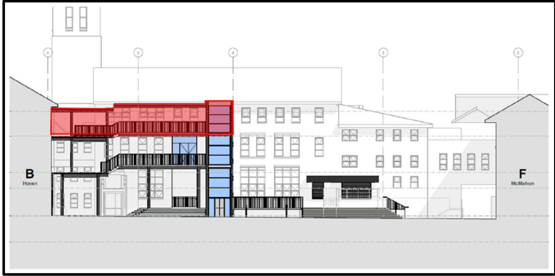
Figure 7 Proposed Internal Courtyard Elevation (Non Conforming Lift/Balcony Shaded Red) (source: DFP Planning Pty Ltd)
