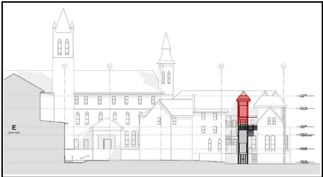
Figure 8 Proposed Rear Elevation of Block A and Block B (Non-Conforming Lift Shaded Red) (source: DFP Planning Pty Ltd)
