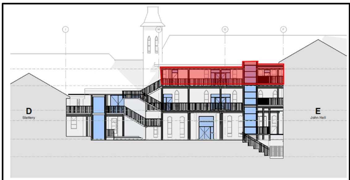
Figure 6 Proposed Internal Courtyard Elevation (Non-Conforming Lift/Balcony Shaded Red) (source: DFP Planning Pty Ltd)
